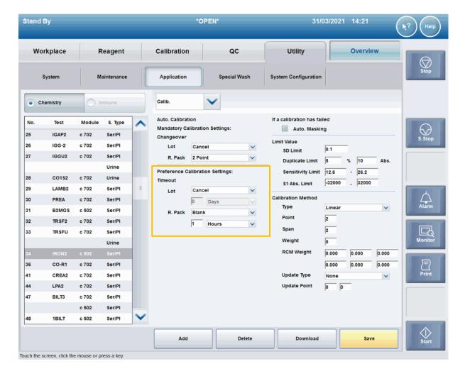
According to the method sheets of IRON2, the calibration recommendation for cassette calibration Timeout is a 2-point calibration every 7 days. After Changing the cassette calibration "Timeout" to "Blank" every "xx" hours, customers are still required to perform a 2-Point calibration manually after 7 days if the cassette is on board for at least 7 days.
